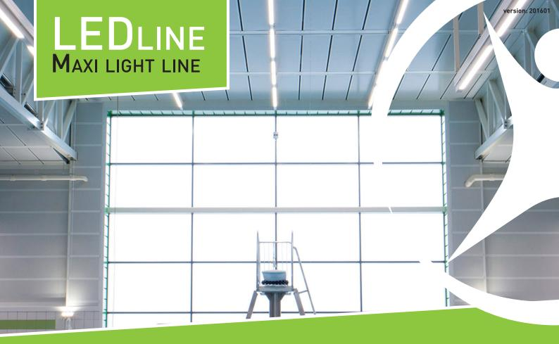
The LEDline Maxi is a multi-functional lighting fixture line with many variations. It is applicable as line lighting in a factory hall or parking garage thanks to the connectivity of the fittings. Available from 30 cm. to 6 metres, which means great lengths can be realised.
